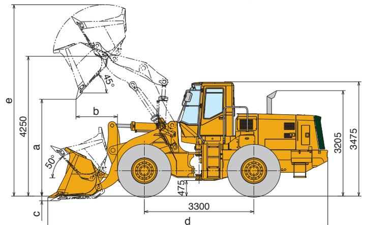
Equipped with GST bucket, 23.5 (L3) tubeless tire and ROPS cab.
